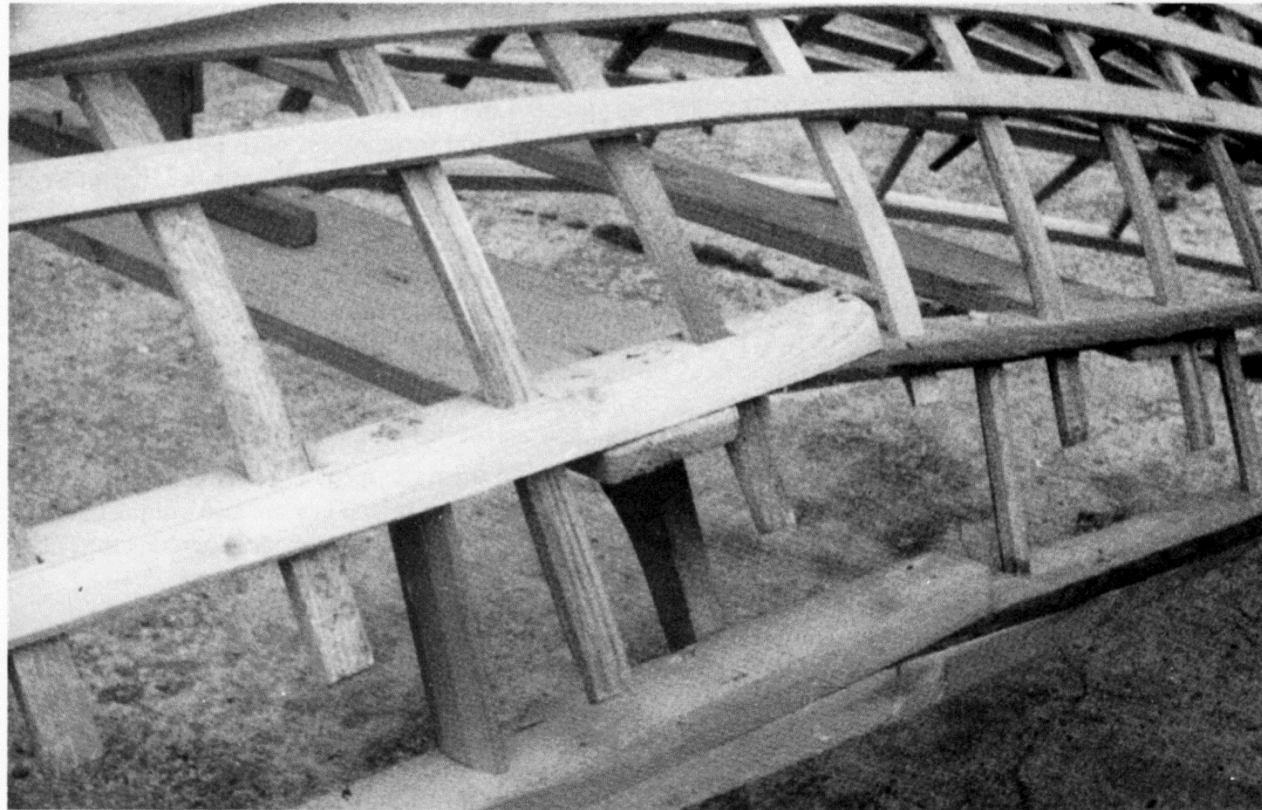
Figure 10.1 Five stages in the building of a curach or navog in Co. Kerry. (Photos: National Museum of Ireland.)
