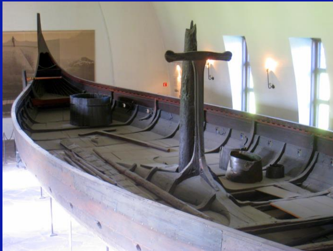
Viking mast step arrangement
