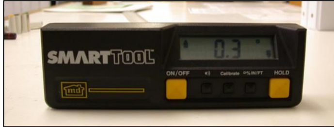
Figure 16 – Digital goniometer (Photo: Filipe Castro).
