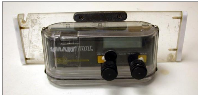
Figure 17 – Dry case for a digital goniometer (Photo: Filipe Castro).
