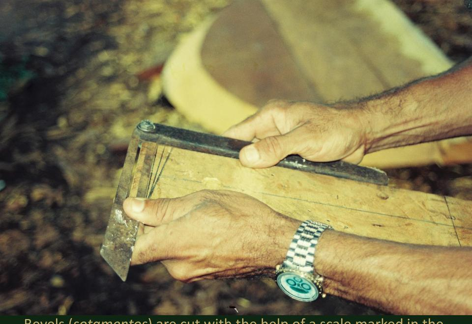
Bevels (sotamentos) are cut with the help of a scale marked in the graminho.
