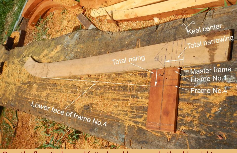
Once the floor timber and futtock molds are ready, the shipwrights define the total rising and narrowing of the turn of the bilge and trace the respective *graminhos*.
