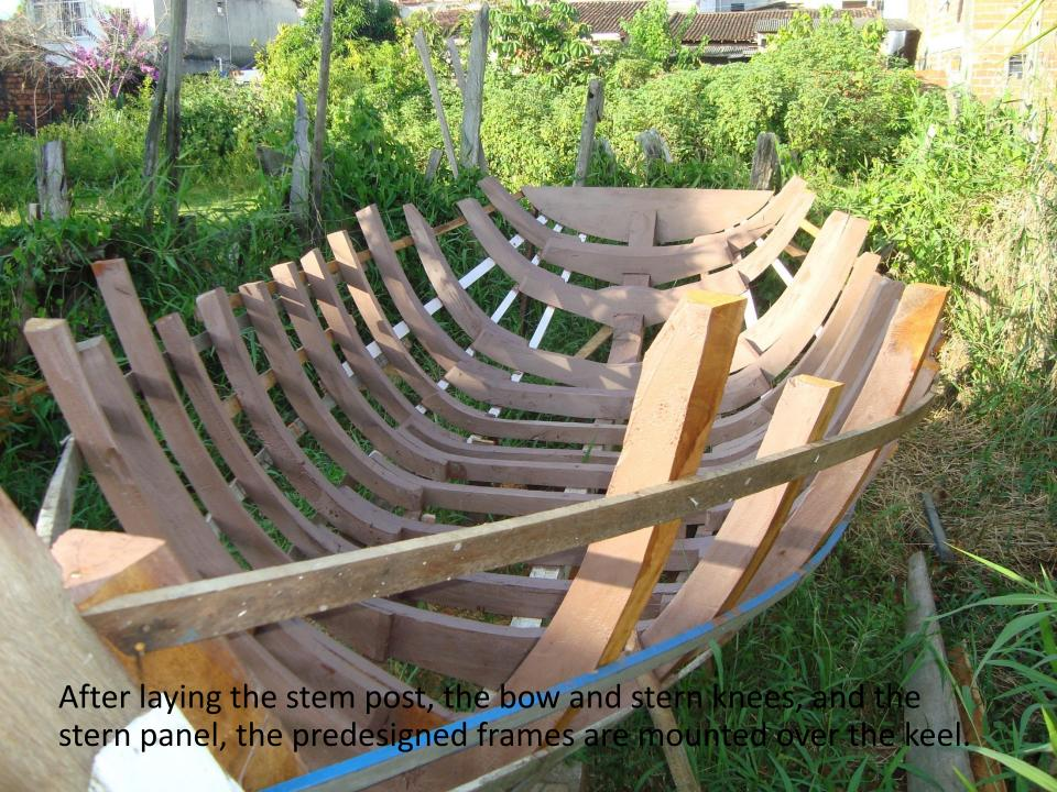
The alignment of the frames is extremely important because once it is done, the keelson is fastened to the keel and the ribbands (*armadouras*) are nailed to the frames in a way that ensures a perfectly symmetrical berth from which the bow and stern frames (*enchimentos*) are shaped.
