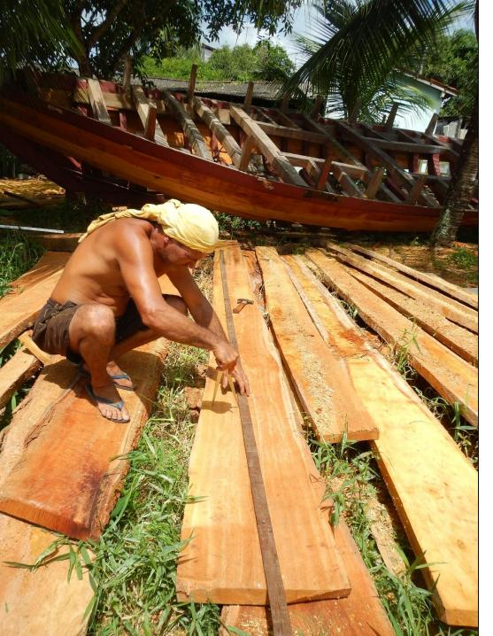
Spiling (fasquilhar) is done with a thin ribband (fasquilha), from which offsets are measured at each frame. The measurements are transferred to the inner face of the plank being shaped.
