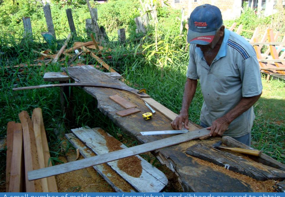
A small number of molds, gauges (*graminhos*), and ribbands are used to obtain – or repeat – a particular hull shape with reasonable accuracy.
