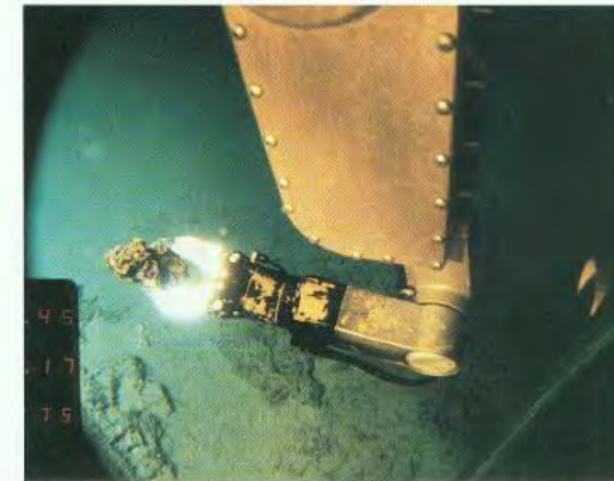
Color fig.25. ROV Jason's robotic claw with small sample in its grasp. Photo: Quest Group, Ltd.
